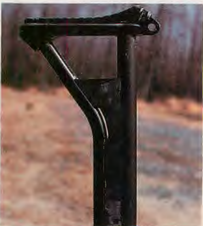
ABOVE: SAW front sight and gas regulator. BELOW: Textured, curved butt pad.
